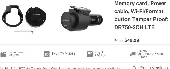
The BlackVue BTC-3A Tamper-Proof Case is a security accessory designed specifically for Blackvue DR750-2CH-LTE and LTE-PLUS series dashcams. It blocks physical access to the microSD card slot, and prevents unplugging the power, and rear camera cables, greatly reducing risks of data tampering. It also limits the angle of rotation of the dashcam ...
